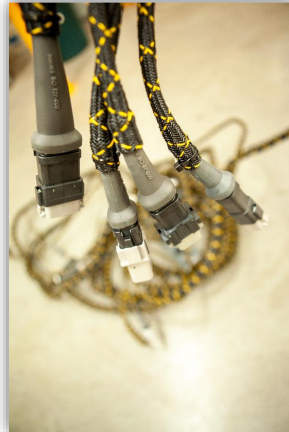
Image 40 - Plugs and Sockets are all environmentally sealed to stop moisture ingress
