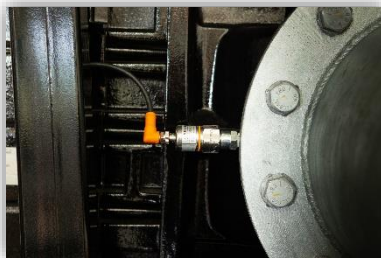
Image 3 – Pressure monitoring allows the operator to monitor the vacuum percentage
