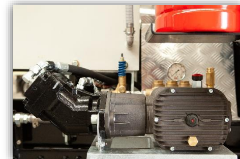
Image 26 - Unloader and safety valves
