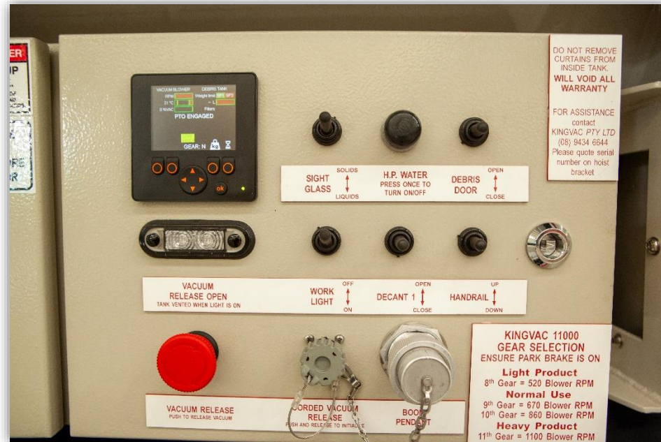
Image 34 - Control system guards against operational errors that would cause damage to the machine
