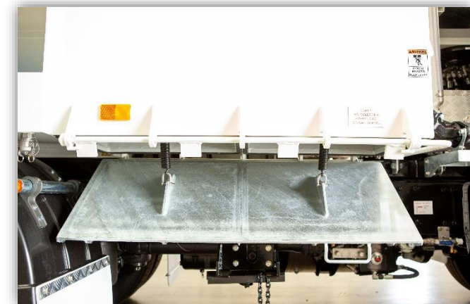
Image 12 - Dropbox for removal of dust
