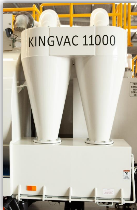
Image 10 - Twin cyclone design in series configuration
