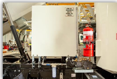
Image 24 - Chassis mounted 700L water tank
