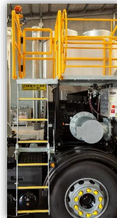
Image 37 - Foldable ladder to platform and stairs to debris tank
