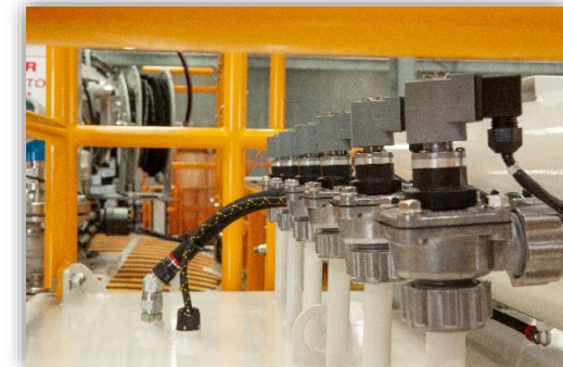
Image 16 - Reverse pulsation system allows constant filter cleaning
