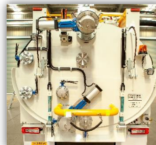
Image 19- Half opening debris door with single function unlock/open and close/lock
