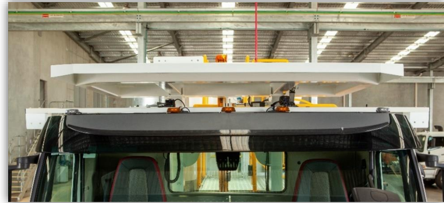
Image 28 - Low profile for aerodynamics and low headroom
