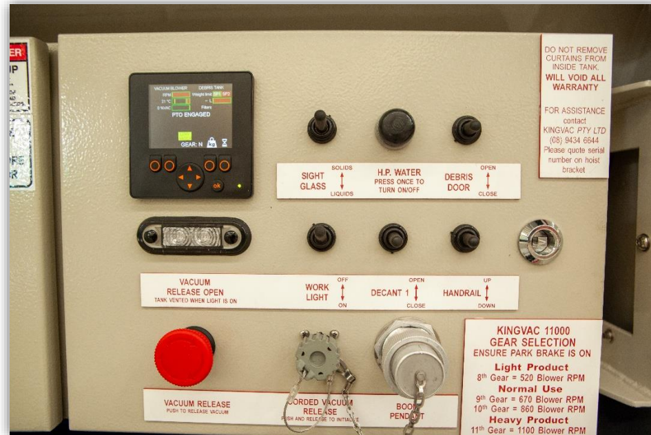
Image 34 - Control system guards against operational errors that would causes damage to the machine
