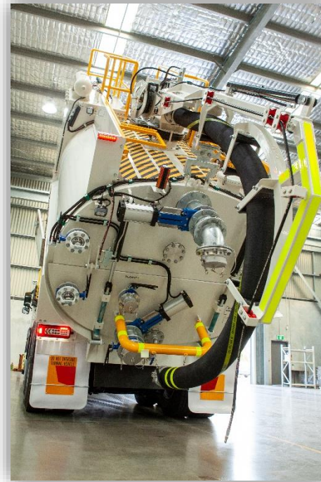
Image 21- Boom allows for easy handling of 6" hose and fittings
