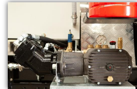
Image 26 - Unloader and safety valves
