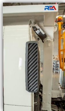
Image 29 - Electric lifting of the canopy allows for tilting the cab
